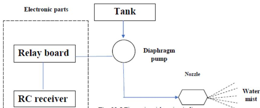
Fig: 11.5 Fire extinguisher circuit diagram
